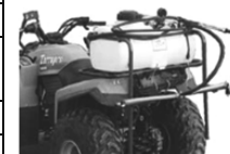
14 GAL Two nozzle 80" swath boom
